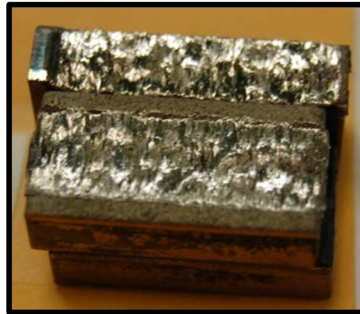
Figure 6. T-800 (Leading Aerospace Coating) Subjected to step-loading using a 5 Ksi and 5,000 cycle interval and ending at 45 Ksi, 5,000 cycles.
