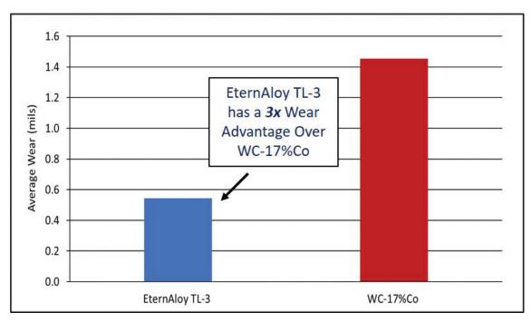
Measured wear after reciprocating tests at 700psi stress, 50 mils (1.3mm) stroke, and frequency oscillation between 25 Hz/50,000 cycles and 1 Hz/20 cycles for 1,000,000 cycles at 600°F (315°C)
