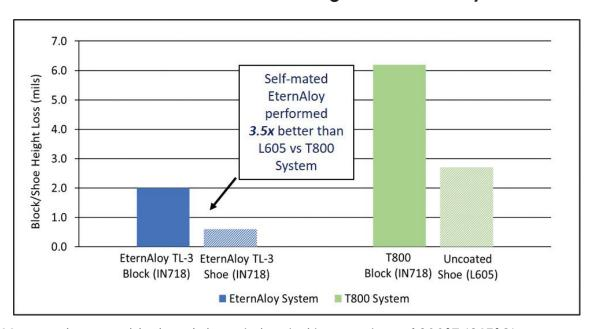
Measured wear on block and shoe at elevated temperature of 600°F (315°C), pressure of 2.5Ksi, displacement of 40 mils (1mm) peak-to-peak, and frequency of 35 Hz for 1,000,000 cycles
