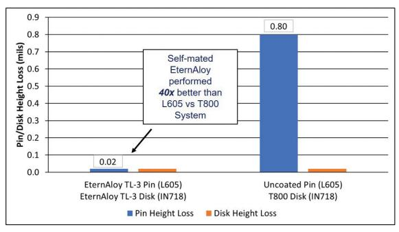
Thermal cycling tests at ~7Ksi and sliding velocity of 2 in/s (50 mm/s) for 19.7K inches (500m) at 150°F(66°C) followed by 19.7K inches (500m) at 550°F(288°C)
