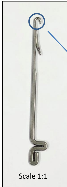
Uncoated used needle showing wear mark in "crook"
